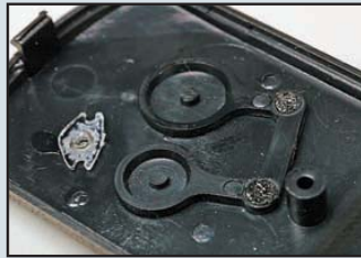
The keyfob case is supplied with the key switch covers mounted as shown here. This assembly must be removed.
