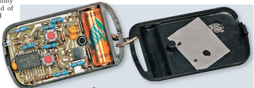
Above: the finished transmitter board inside its keyfob-style plastic case. Power comes from a 12V A23 car alarm battery. Note how the keyswitch covers are mounted on the lid, using a 20 × 24mm silicone washer – see text.
